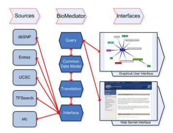
**Fig. 2.** Overview diagram of SNPit [15]. The system is comprised of three sections: data sources related to SNP annotation, the BioMediator federated data integration system, and both a graphical user and web servlet interface.
