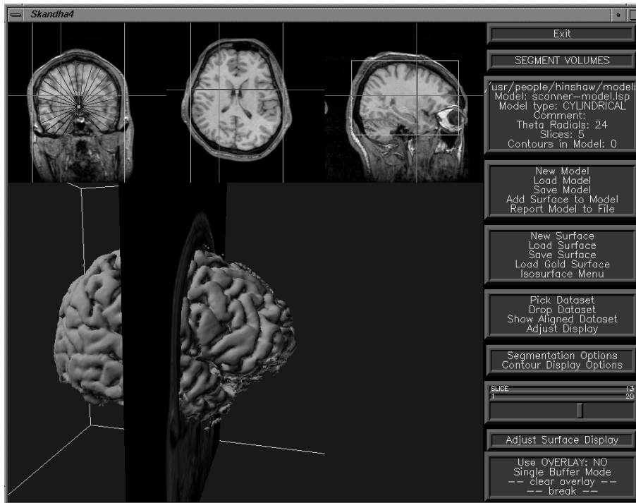
Figure 2: The segmentation interface. Slices through the MR volume are shown at top, with radials from a fitted model displayed on the coronal slice. Bottom left shows an extracted isosurface.
